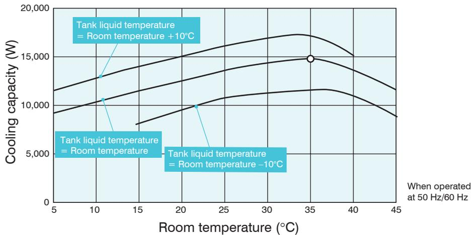
1. The mark "O" shows the standard point. (Room temperature: 35°C, Tank fluid temperature: 35°C, Oil used: ISO VG32 (water in the case of AKJ1509), 1 atm)
