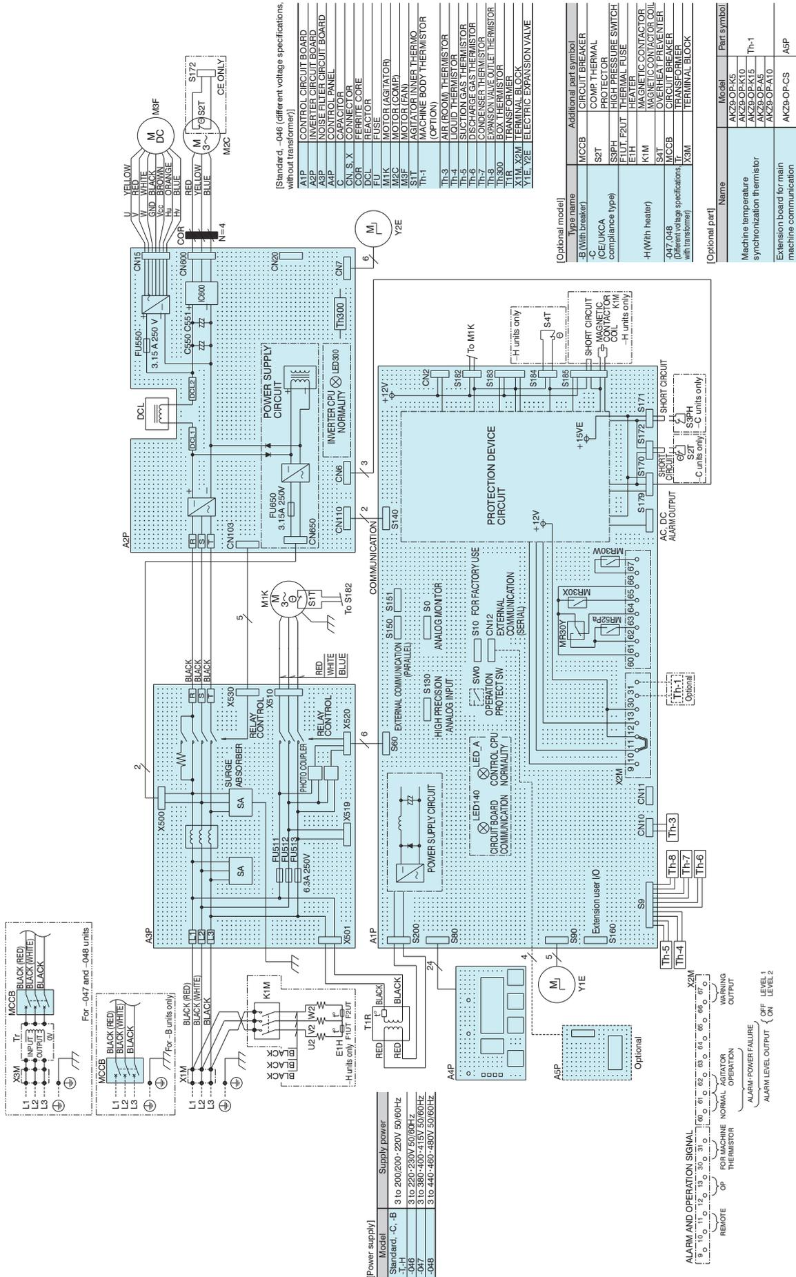
Electric Wiring Diagram (representative model of AKJ9W Series)
