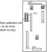
Part layout diagram for KC-6-10, viewing the panel from the rear.
