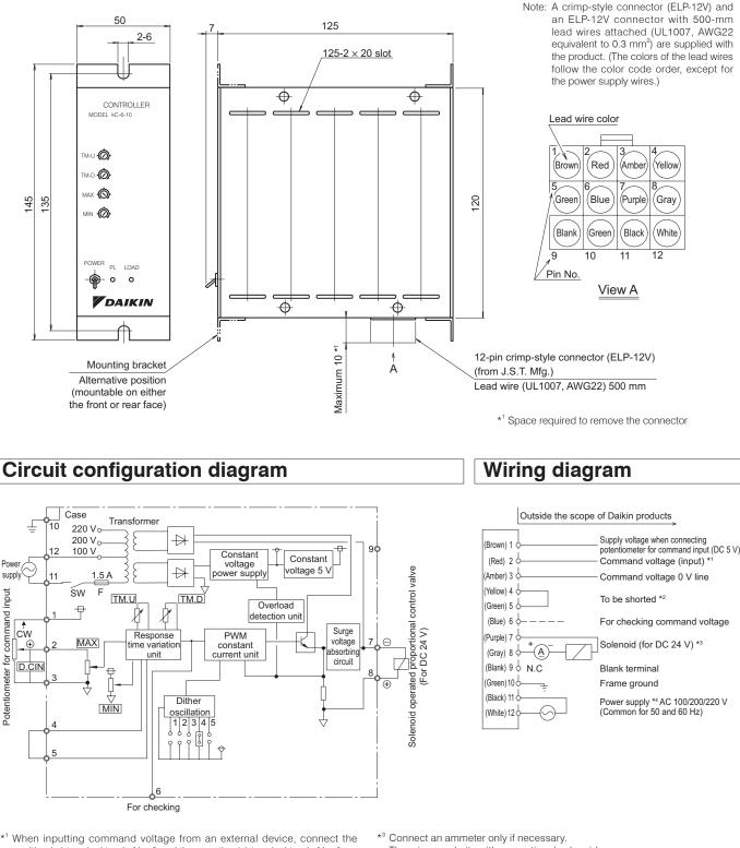
positive (+) terminal to pin No. 2 and the negative (-) terminal to pin No. 3. When connecting a potentiometer for command input, follow the sample wiring below
