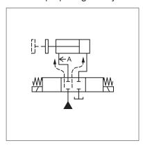
The cylinder may be self-propelled in very slow speed due to leakage at a directional control valve in a circuit as shown in the figure to the left where the load to the cylinder is light and the pressure within the line is retained.
