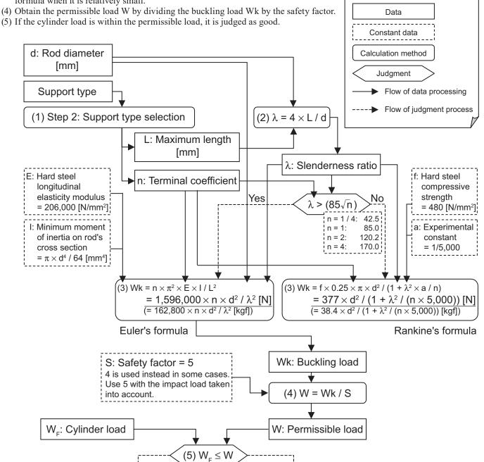
Figure: Flow of buckling calculation
