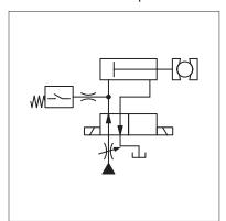
The pressure switch may malfunction due to surge pressure on excitation of a solenoid valve in a circuit as shown in the figure to the left.
