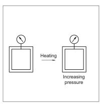
Heating hydraulic fluid within an airtight container will expand the fluid and increase the pressure.
