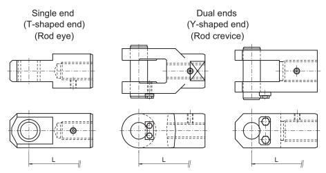
Figure: Example of end bracket
