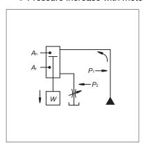
Use of a meter-out throttle as shown in the figure to the left increases the pressure. Especially when the cylinder is directed downward and there is a hanging load however, abnormal pressure at the rod side may occur.
