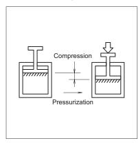
Hydraulic fluid has a small compressibility compared to air but its volume will be reduced by 1% on application of a pressure of 20 MPa {200 kgf/cm²}. For this reason, sudden switching of a solenoid valve may cause a shock.
